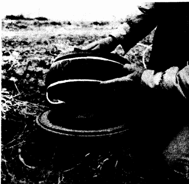
Figure 8.7 Improved USDA inflatable pneumatic O-ring valve. (From Haise et al., 1980.)
